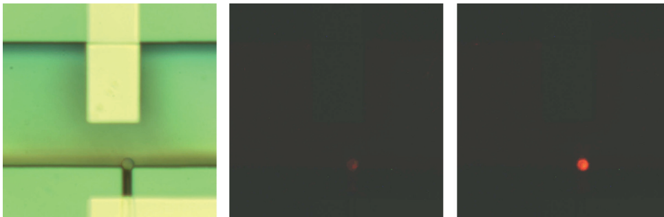
Figure 7-5: Light image of trapped yeast cell. PI response after 6 pulses and after 7 pulses of 10 \mu\text{s} and electric field strength of 9 \text{ kV}\cdot\text{cm}^{-1} .
